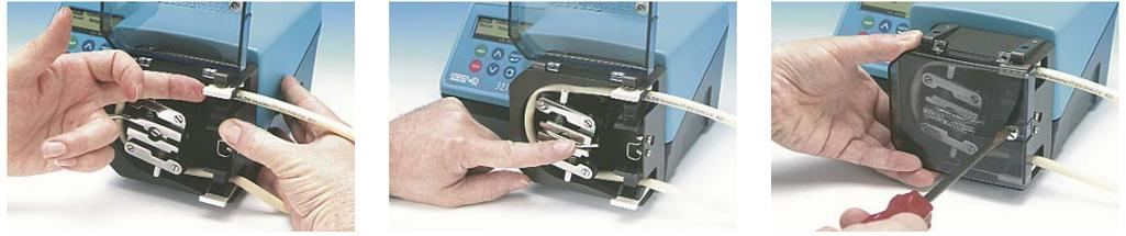
The tube clamps can accommodate various tube diameters by pushing in, or pulling out, the grip bars within the clamp. Set the clamps to apply the minimum necessary pressure to the tubing.
