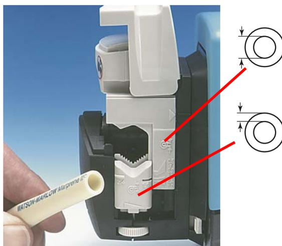
Set the tube clamps to the correct tube size. The track must be fully open. Align the scale on both sides of the pumphead.
