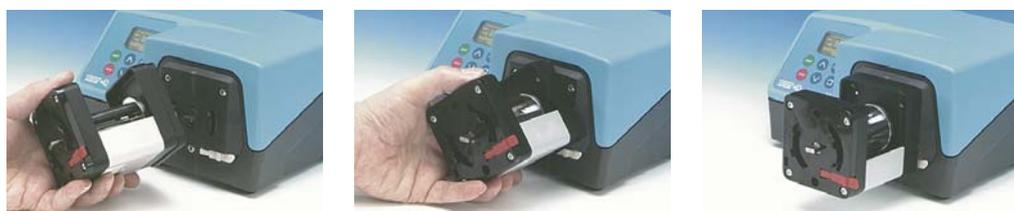
Engage the pumphead drive slot with the end of the pump drive shaft. Continue to align the pumphead until the bayonet engages with the mounting plate. Turn the pumphead clockwise until it locks into an upright position.
