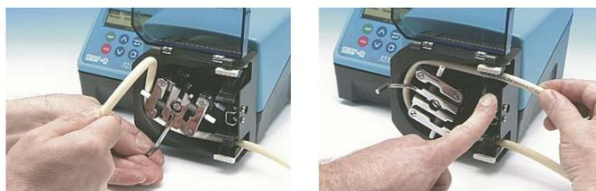
When the tube has gone round the pump track fit the other end of the tubing into the clamp. Check that the tubing has fitted naturally against the track for best tube life. Release the clamps and adjust the tubing if it is slack, twisted, or stretched.
