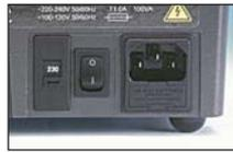
The voltage selector is mounted in the switchplate at the rear of the pump. Set the voltage selector to 115V for 100-120V 50/60Hz supplies or 230V for 200-240V 50/60Hz supplies. Always check the voltage selector switch before connecting the mains supply. Make suitable connection to an earthed, single-phase mains electricity supply. To comply with Safety Standards, the mains plug must be a separable plug (not a locking type).
