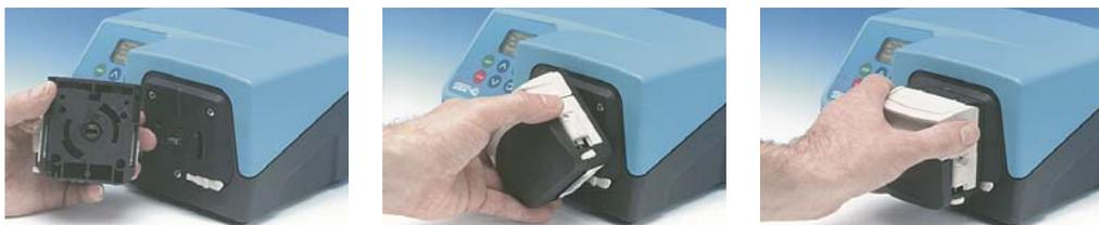
Engage the pumphead drive slot with the end of the pump drive shaft. Continue to align the pumphead until the bayonet engages with the mounting plate. Turn the pumphead clockwise until it locks into an upright position.
