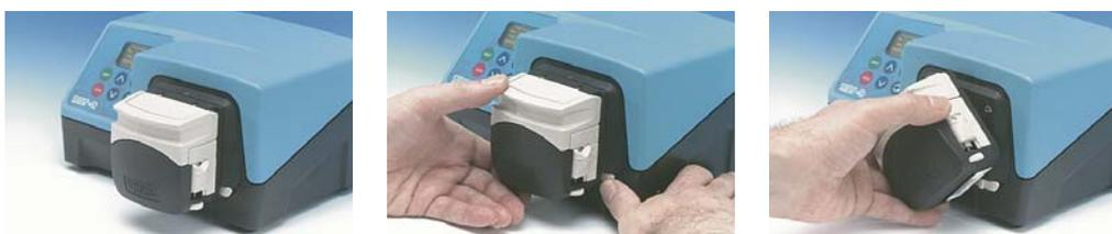
Push the locking lever back and turn the pumphead anti-clockwise until it is free from the mounting plate.
