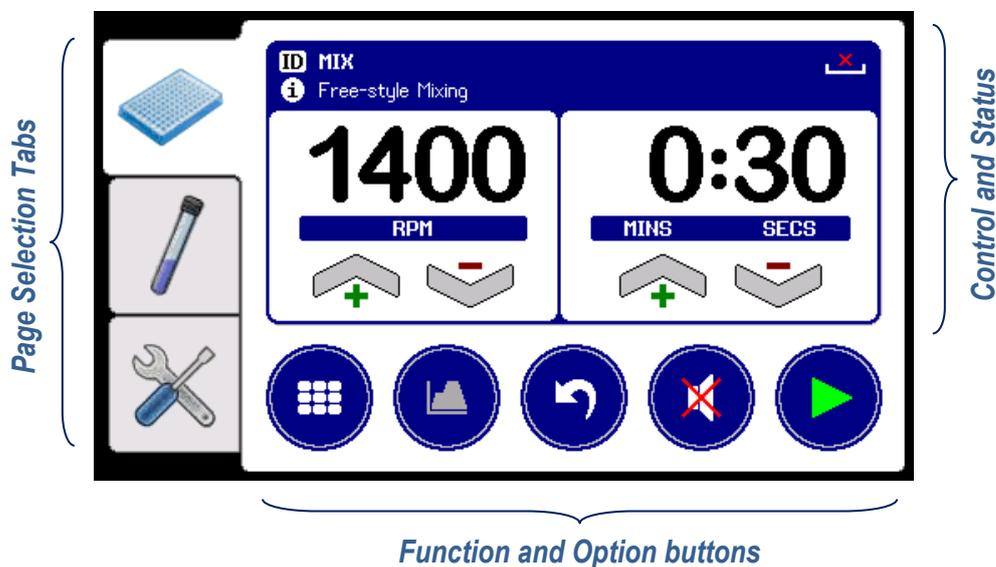
The Co-mix is designed to allow simultaneous operation of both the plate mixer and tube vortexer, by providing easy mode switching using the three page selection tabs shown in Table 4.
