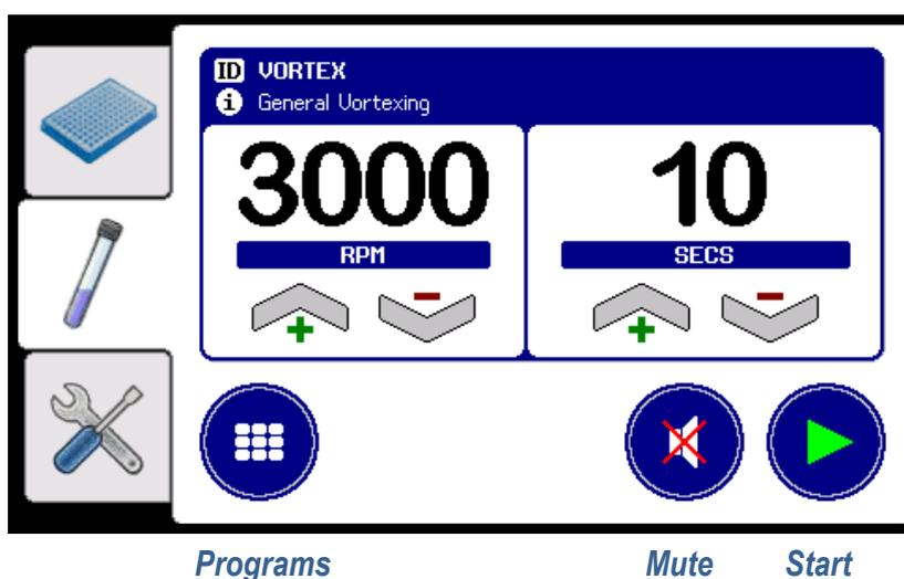
To vortex a tube, simply press the tube down onto the centre of the vortexer pad and vortexing will automatically start at the programmed speed.
