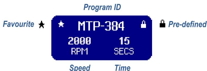
To load a program, use the **Home** button to jump to the top of the program grid list or the **Next** and **Previous** buttons to scroll through the list to highlight the desired program, and then press the **Accept** button.
