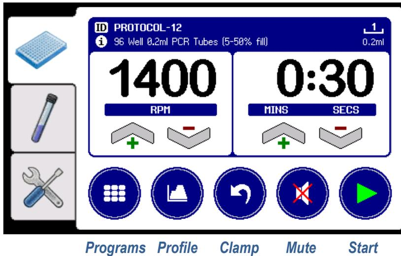
Once **Unlocked**, the **Increase** and **Decrease** buttons can be used whilst the mixer is running to fine tune the mixing performance for the particular plate type, sample solution and fill volume being used. Any changes to these parameters are automatically saved to memory for next time.
