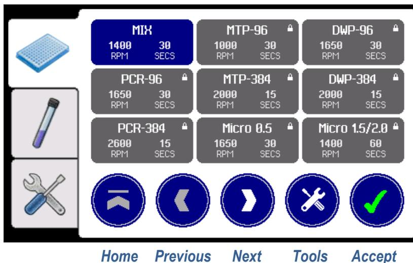
Each program grid button shows the program’s ID and the assigned speed and time parameters.
