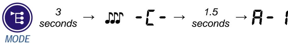
Next use the MODE button to step through the setting options (A, C and H), and the UP and DOWN buttons to change the setting value (0, 1 or 2).
