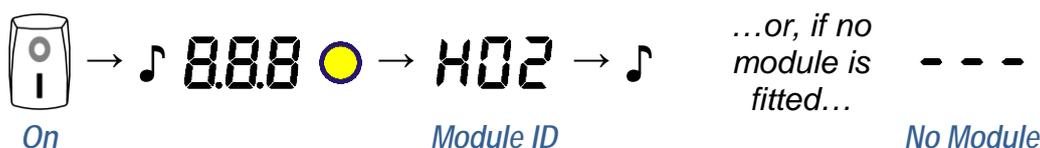
If no module is fitted, or it is not fully screwed down (see section 6.2), the unit will not display a Module ID and no further actions can be performed until the module is correctly affixed.
