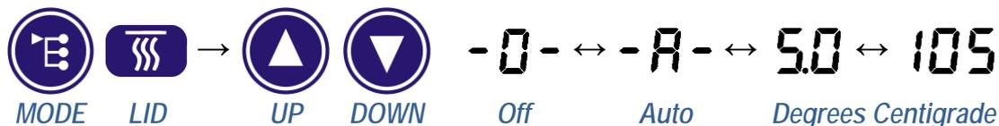
In Auto mode, the lid automatically adjusts its temperature to be higher than the sample block temperature, thus preventing condensation from forming on the caps of the sample vessels. In Off mode, the lid heater is disabled.
