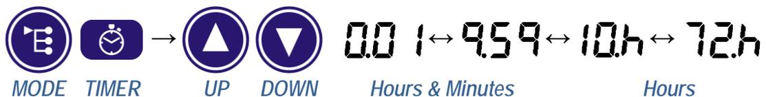
**i** The timer duration can only be changed when the TIMER display mode is selected and the timer it is not running (i.e. the TIMER status LED is off). The new time setting is stored within the Heated Module when the START button is next pressed.
