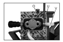
Detach the coupling of the connection tube (V) to the other side of the pump at the valve head (O).
