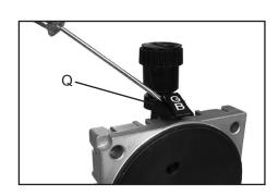
→ Open the hinged cover of the connection fastener (Q) with a slotted screwdriver.
