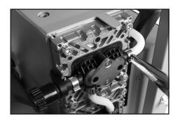
Affix the connection tube (V) to the other side of the pump at the valve head (O).
