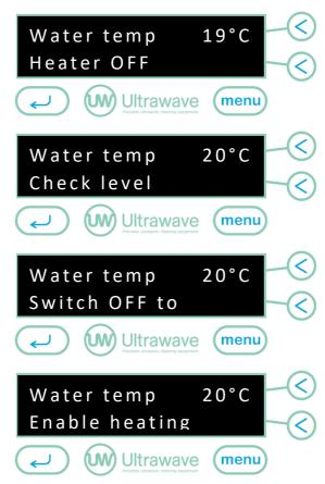
To continue using your Sanitiser Series ultrasonic bath, refill with liquid up to the level sensor, switch the unit off and on again.
