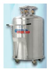
All Cryostors are equiped with a safety dispensing head incorporating fill, vent and dispense valves, safety reliefs, pressure gauge and an integral pressure build vapouriser with automatic pressure regulation.
