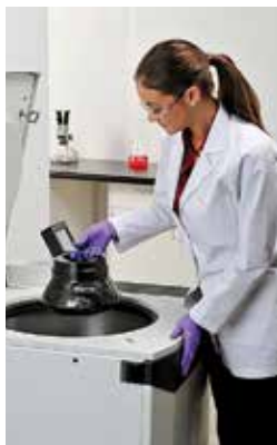
1. Place rotor into the centrifuge chamber
