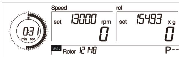
Fig. 5.15: Preselection of a rotor
