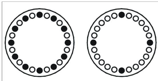
*Fig. 5.8: Permissible loading of the angle rotor*
