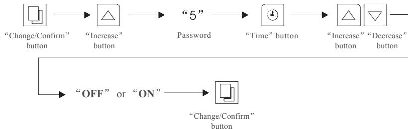
1. When the above setting is finished, press the “Start/Hold” button and the equipment will run according to the designed program.
