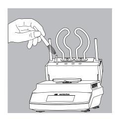
4) Clean the heating element and temperature sensor with a weak solvent such as ethanol.
