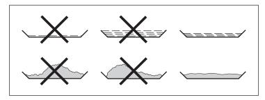
While preparing substances for measurement, no processes may be used that generate heat. The heat generated may result in a loss of moisture prior to the measurement.
