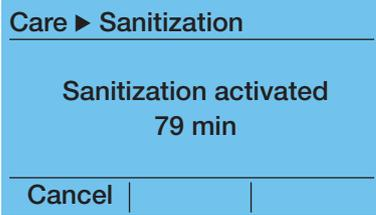
▷ Sanitization is performed. The remaining time is shown on the display.
