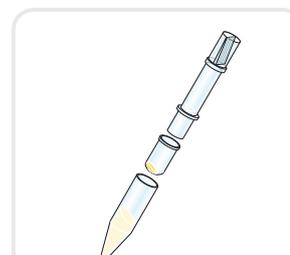
Direct pipette recovery or choice of reverse spinning concentrate into sample cap
