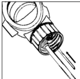
Insert the recirculation tube firmly into the recirculation opening in the valve block.
