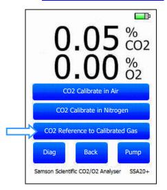
Connect a calibration gas supply with pressure set no higher than 0.3L/min and turn on the supply
