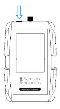
After being turned on, the SSA-20+ will start up within 3 seconds and the current  $CO_2$  and  $O_2$  measured values will be displayed.
