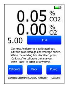
When the reading has stabilised press Calibrate and the SSA-20+ will adjust the measured level to match the calibration gas value
