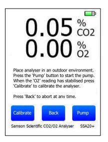
When the reading has stabilised, press Calibrate and the SSA-20+ will adjust the measured O2 level to 20.9%
