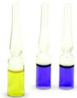
offers regular biological indicators as well as self contained biological indicators. Simply place the SCBI into the autoclave, remove after cycle end, crush the cap (or squeeze the side for Mini SCBIs) and incubate for 24 hours. A negative result ensures the micro-organism within has been destroyed and guarantees sterility of the process.
