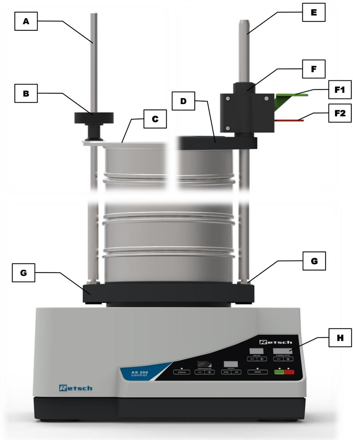
Fig. 8: Front view of the device with different sieve clamping units
