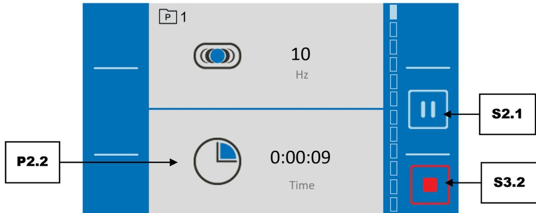
Fig. 27: Programme mode after starting the grinding process
