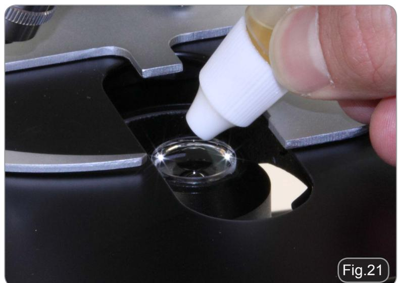
4. Reposition the slide and raise the condenser until the oil on the lens of the condenser is in contact with the slide.
