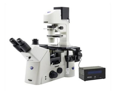
Laboratory inverted microscope for research applications.
