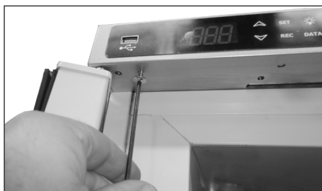
42....and remember the screw close to the top door pivot is mounted in hole nr.2 inwards, to ensure sufficient space between the screw and the door end-cap during mounting
