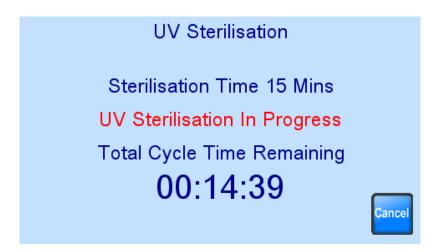
If the safety screen is removed or the button is pressed the cycle will terminate and the normal running screen will be displayed
