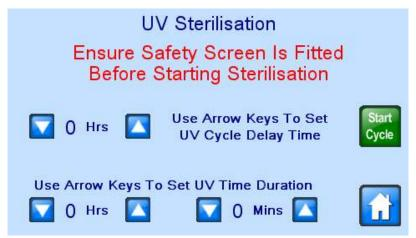
The safety screen is interlocked with the UV sterilisation cycle and the cycle will not run if it is not fitted. Use the arrow keys to set the sterilisation time and cycle start delay if required.
