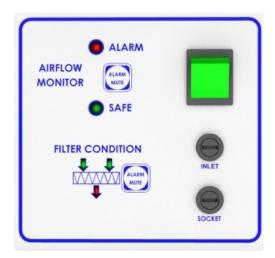
The cabinet is started by the illuminated rocker switch on the control panel. When the fan reaches normal operating speed the green 'SAFE' warning light will indicate that the cabinet is ready for use. If the red 'ALARM 'indicator flashes and the alarm beeper sounds, the pre-filters may require changing (See section 4 for details).
