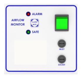
The cabinet is started by the illuminated rocker switch on the control panel. When the fan reaches normal operating speed the 'SAFE' warning light will come on and the cabinet is ready for use. If the 'ALARM 'indicator lights and the alarm beeper sounds, the airflow has reduced to below a safe working limit (<0.3m/sec), pre-filters may require changing (See section 4 for details of filter changing).
