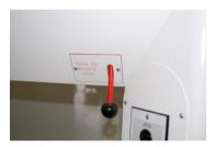
At all times make sure to close the sash fully, thus providing maximum protection to the user. If large equipment is to be loaded into the fume cupboard chamber, the sash can be raised further by pushing the sash restrictor knob upwards, once the sash is lowered the sash stop will automatically reset.
