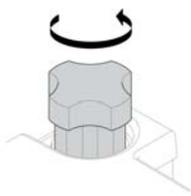
1-Using the tool, unscrew the sanitation port cap.
