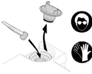
2-Remove the plug and insert the tablet in the port.
