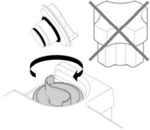
3-Screw the plug back: make sure the o-ring is in place.
