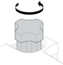
1-Using the tool, unscrew the sanitation port cap.
