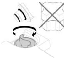
7-Screw the plug back and put the system in Tank filling by pressing twice
