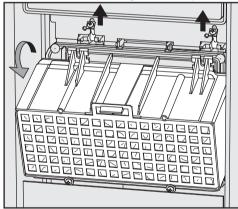
■ Remove the coarse filter housing.
