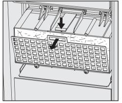
■ Remove the filter mesh at the front of the drying unit.
