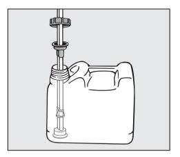
Insert the siphon tube into the container opening and screw it into place. Make sure to observe the color coding.
