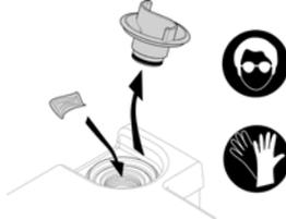
2-Remove the plug and insert the tablet in the port.
