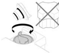
7-Screw the plug back and put the system in Tank filling by pressing twice
