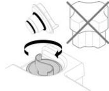
3-Screw the plug back: make sure the o-ring is in place.
