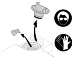
6-Unscrew the plug and remove the empty pouch from the cleaning port.
