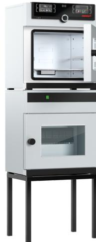
The direct contact between the load and the heatable and removable thermoshelves in the chamber of the Memmert vacuum oven VO ensures rapid and uniform temperature control of food, cosmetics, watches, books, PCBs or injection moulds, without the loss of heat.
