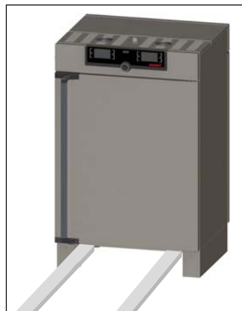
Fig. 8 Transporting by forklift
