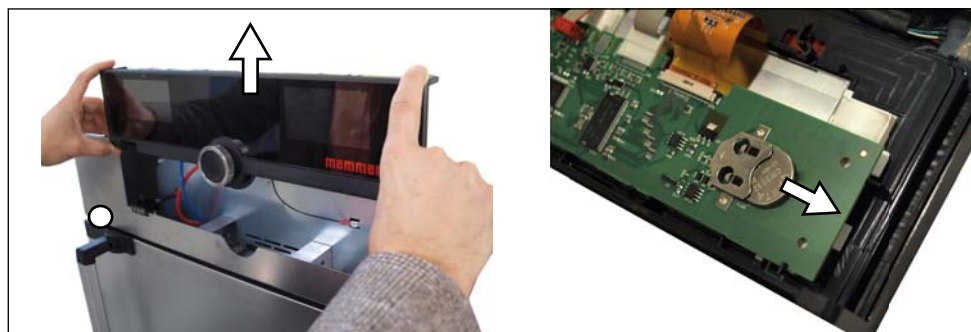
Fig. 31 Removing the lithium battery
