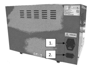
Figure 2 – LyoDry Benchtop Pro Rear connections.
