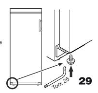
**29.** Screw the screw into the pin again and tighten.
