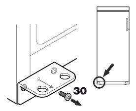
**30.** Remove middle screw from hinge bracket. This screw is no longer needed.
