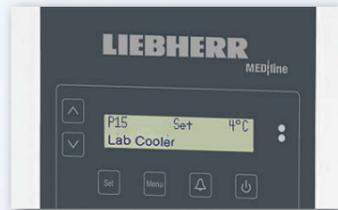
The **Profi electronic controller** has an integrated data memory for **temperature recording**.
