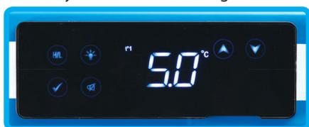
The touch screen controller is completely flat so can be thoroughly cleaned and disinfected as there are no raised buttons to collect dirt and germs. The controller displays, alarms and records minimum and maximum temperatures for both temperature probes. Like a mobile phone touch screen it locks after 30 seconds to ensure that buttons can't be activated accidentally.
