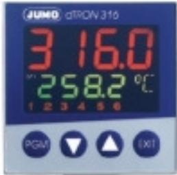
The temperature is accurately controlled by a Jumo dTRON 316 microprocessor temperature controller. The controller uses the signal from a PT100 sensor located in the chamber to control the current supplied to the heaters. The temperature can be easily adjusted (see section 3 for full details). A separate digital temperature display unit sets the over temperature safety cutout. This is normally set to 2°C above the required chamber temperature.
