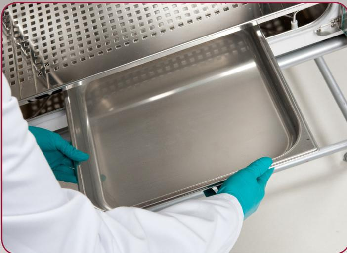
Ensure the water tray is empty of all water, make sure both the inner and outer door are closed securely
