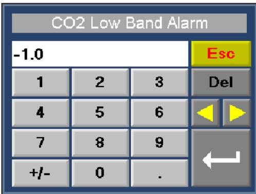
Use the keypad to change the low alarm threshold.
