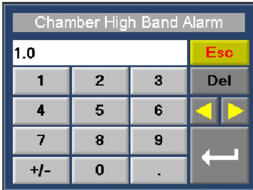
Use the keypad to change the high alarm threshold.
