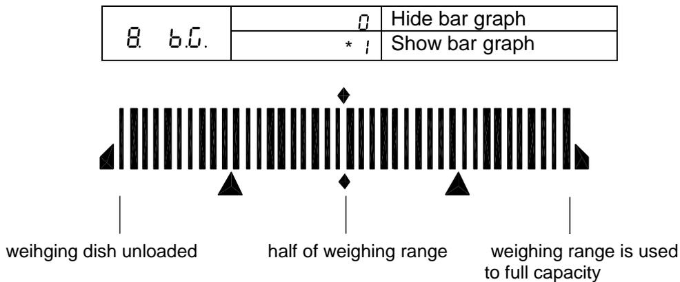
The weighing range of the balance is divided into 40 graphic cuboids. Zero (0) will appear on the graphic display if there is no weighing value on the balance. 20 graphic cuboids are displayed if the balance is loaded up to one half of its weighing range.
