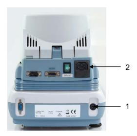
Power is supplied to the balance via the external power unit. The stated voltage value must be the same as the local voltage. Only use original KERN mains adapters. Using other makes requires consent by KERN. After connection to the power supply the balance will carry out a self-test. The balance changes into stand-by mode.
