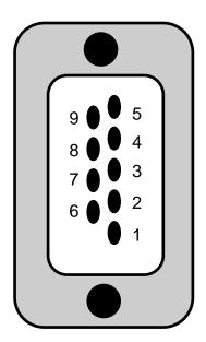
Pin 2: Tx Signal Pin 3: Rx Signal Pin 5: GND
