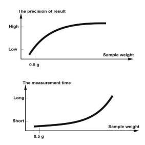
However, the heavier the originally weighted in quantity, the more accurate a result.
