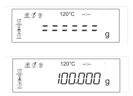
After successful adjustment the balance automatically returns to weighing mode, "100,000 g" will be displayed. Take away adjustment weight.
