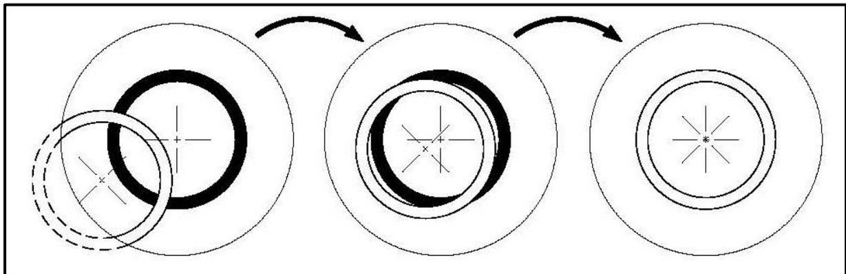
Depending on the preferences of the user, using a green filter can produce a more effective and pleasant image. To achieve this, the green filter must be screwed onto the underside of the PH condenser.
