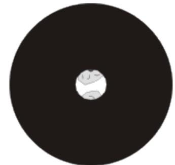
4. Open the field diaphragm until it just disappears out of the field of view.
