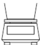
⇒ Place the empty weighing container on the weighing plate
