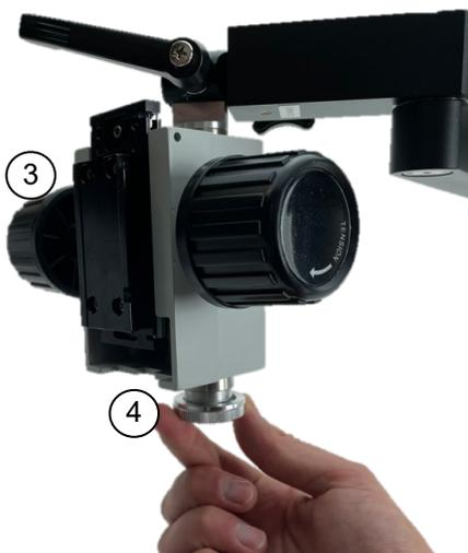
Secure the holder for the microscope head (3) with the knurled screw (4) to prevent it from falling down.
