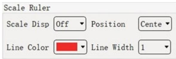
Display of the scale (Scale Disp): If you switch to On, the scale is displayed; if you switch to Off, the scale is closed.
