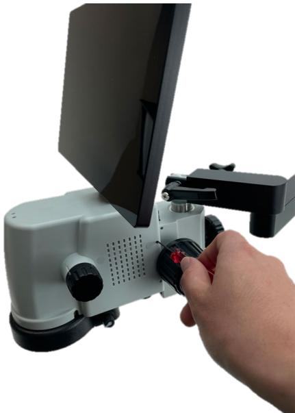
To attach the microscope head to the stand, tighten the screws (2x) on the outside of the housing using the Allen key supplied.
