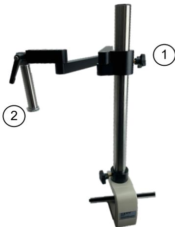
Insert the movable arm into the microscope column and tighten the locking screw (1). Now loosen the knurled screw (2) and insert the holder for the microscope head into the shaft.
