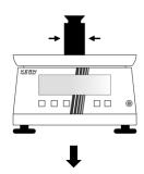
⇒ Place the calibration weight in the centre of the weighing plate
