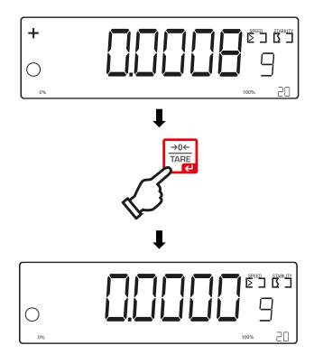
□ Unload the scales and check the stability indicator
