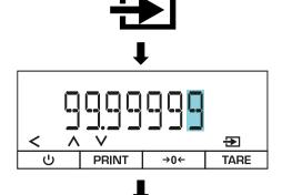
⇒ Enter the value for the specific density of the auxiliary medium (unit g / cm³; for numerical input, see Chap. 3.2.2)
