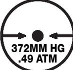
Indicates the acceptable lowest barometric pressure conditions in which this unit can be shipped.
