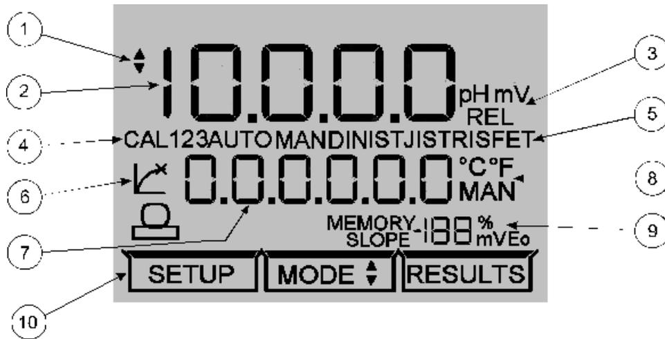
1. Symbol – displayed during set-up of instrument parameters.
