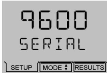
The secondary display will show BAUD and will then scroll SERIAL PORT BAUD RATE after 10 seconds.
