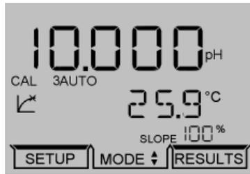
If a successful 1 point calibration has been performed the secondary display will momentarily show CAL OK. The slope value from the calibration will be displayed. The instrument will then update the display.
