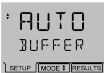
The secondary display will show BUFFER and will then scroll BUFFER TYPE after 10 seconds. Select the type of buffer from the options available by scrolling through the list using the Up/Down arrows – AUTO, MAN, JIS, NIST or DIN. (AUTO relates to the Jenway buffer types supplied with the instrument).
