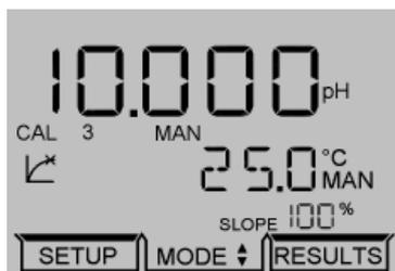
If a successful 1 point calibration has been performed the secondary display will momentarily show CAL OK. The instrument will then update the display.
