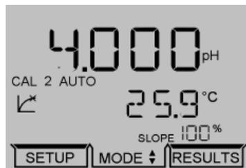
If a successful calibration has been performed the secondary display will momentarily show CAL OK. The instrument will then update the display. The display will then show the next part of the calibration sequence if a 3 point calibration has been selected. If a 2 point calibration only is required the instrument will return to the main measuring screen.
