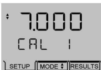
with the first digit of the value flashing. Adjustment of the flashing digit can be made using the Up/Down arrow keys. The Left/Right arrow keys are used to select the next adjusting digit which will flash when selected. Once the full reading has been adjusted to the correct value, press the STO key. If a 1 point calibration only is being performed the instrument display will update and show the pH Resolution set up menu.
