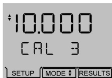
The correct values should be entered and saved as for the 1 point calibration. When all chosen buffer types have been entered and confirmed the instrument display will update to show the next set up menu option.
