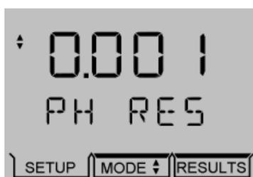
The secondary display will show PH RES and will then scroll PH RESOLUTION after 10 seconds.
