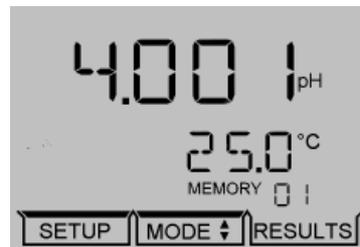
The Up arrow increments the memory index, the Down arrow decrements the memory index.
