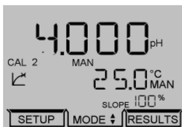
If a successful calibration has been performed the secondary display will momentarily show CAL OK. The instrument will then update the display. The display will then show the next part of the calibration sequence if a 3 point calibration has been selected. If a 2 point calibration only is required the instrument will return to the main measuring screen.
