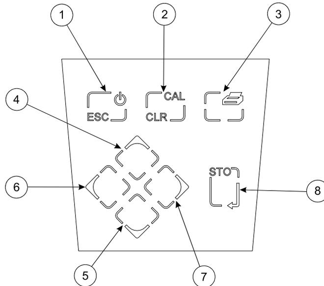
1. ESC used to switch the instrument on and to place into standby mode (only if power supply lead remains connected to the instrument). Also used to escape/exit a mode.
