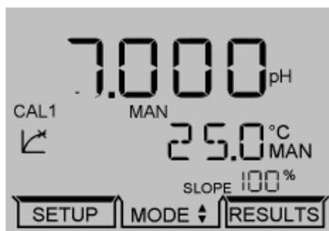
If a successful 1 point calibration has been performed the secondary display will momentarily show CAL OK. The instrument will then update the display. The display will then show the next part of the calibration sequence if a 2 and/or 3 point calibration has been selected. If a 1 point calibration only is required the instrument will return to the main measuring screen. Eo is shown on the status display
