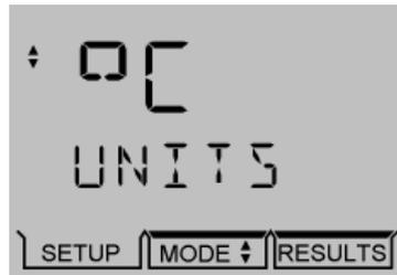
The secondary display will show UNITS and will then scroll TEMPERATURE UNITS after 10 seconds.
