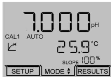
If a successful 1 point calibration has been performed the secondary display will momentarily show CAL OK. The instrument will then update the display. The display will then show the next part of the calibration sequence if a 2 and 3 point calibration has been selected. If a 1 point calibration only is required the instrument will display the Eo value on the status screen and then return to the main measuring screen.
