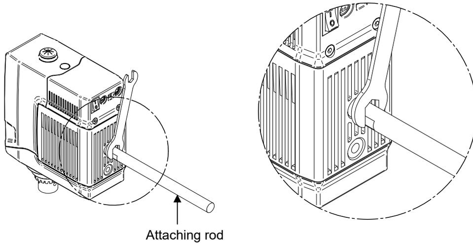
As above, one basic shaft must be turned on the right and fixed it tight by using spanner 13mm. In case of dial stand use, it must be connected to the specialized attaching rod.
