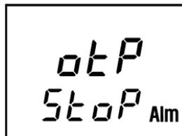
전 Turn off the machine and make it cool for a while. And re-operating. When the cooling time is not enough protect function can be re-activate.
