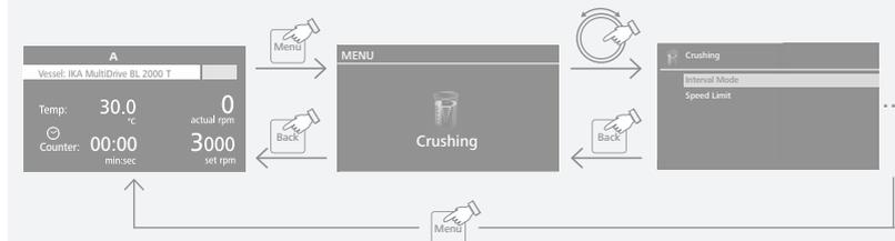
**Note:** If you press the “Menu” button, the system skips directly back to the working screen.
